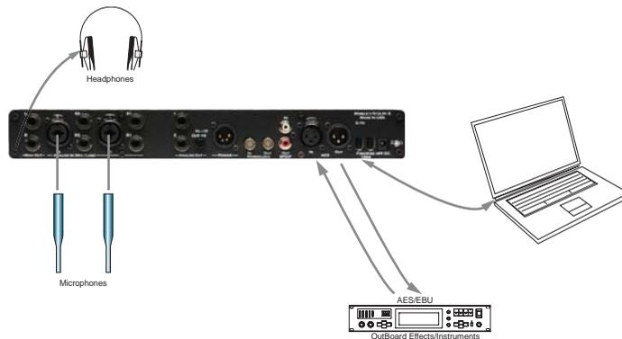
Figure 39: Example ULN-2 Setup
